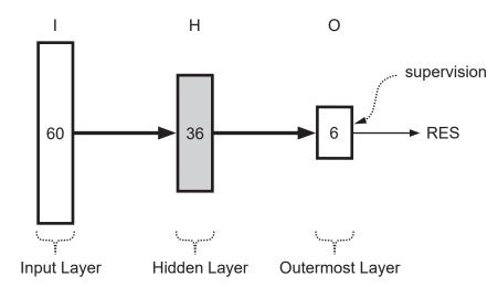
The neural network in the block diagram contains 60 nodes in the input layer (block I), 36 nodes in the hidden layer (block H) and 6 nodes in the outermost layer (block O). The solid black arrows indicate that *all* nodes in one layer are feeding *all* nodes in the successive layer. In particular, the value RES is calculated by using all nodes in O.
